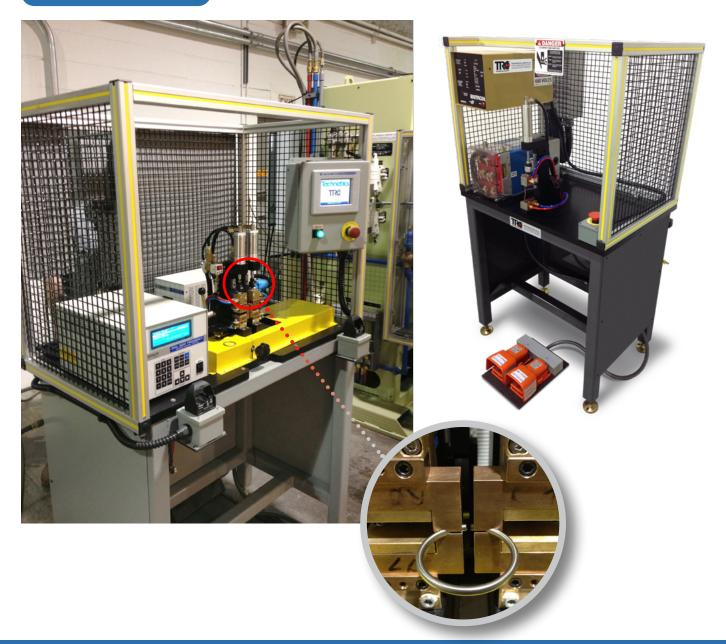
**TRC Fine Spot Welders** are custom designed to weld your particular product and are built to your manufacturing specifications. These welders are uniquely suited for very small applications such as battery pack/terminals, electronic components such as capacitors and resistors, cross wire welding, and many other applications.
