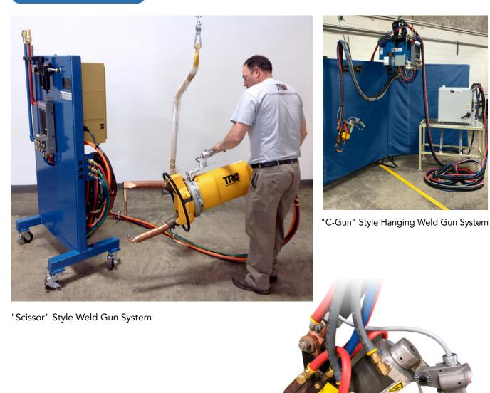
**TRC Portable Weld Gun Stations** are offered in either a manual **Trans-Gun** design or a **Hanging Gun** style. These types of welding systems are best suited for applications where the welding machine needs to be brought to the work. Common applications for **Manual Weld Guns** include door panels, large weldments, or other products that are too large for an operator to manipulate. These systems are designed to fit your application with custom throat heights, depths, arm designs, etc.
