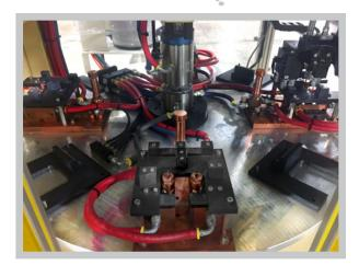
**TRC** designs custom automatic Indexing Welding Systems for spot welding, projection nut welding, and projection stud welding.
