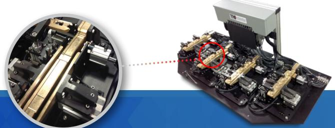
Accurate, precise, and repeatable tooling is a requirement for high volume robotically welded assemblies. **TRC** has the design capabilities, machining capabilities, assembly experts, and over-all experience needed to provide weld tooling for automated applications. We can supply tooling that comes complete with Control Packages, Sensors for all parts, motion, Poke-yokes, and Change-out Tools.
