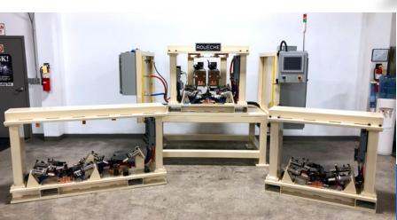
**TRC Flex Weld Stations** are designed to accommodate multiple, interchangeable welding applications that allows you the ability to have advanced controls while still meeting your budgetary requirements. If you have multiple, custom welding applications that are of low to moderate volume – from 20,000-500,000 pieces per year – then this system is for you!
